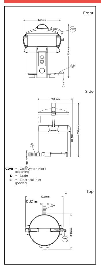
Electric Supply voltage: 220-240 V/1N ph/50/60 Hz Electrical power, max: 0.25 kW 0.25 kW **Total Watts:** Key Information: External dimensions, Width: 424 mm External dimensions, 390 mm Depth: External dimensions, 590 mm Height: **Shipping weight:** 26 kg
